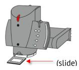
A slide drawer is located on the underside of the camera. When a slide is inserted in to the slide drawer, it is automatically recognised and projected.
